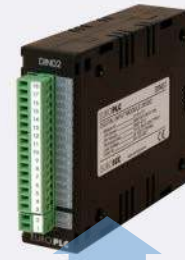
M2.DIO.01 Digital input-output module 16 digital inputs 24 VAC 8 digital inputs 24 VDC 8 transistor outputs
