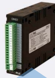
M2.FNM.02 4 digital inputs 24VDC 4 digital transistor outputs 3 analog inputs, 1 analog output
